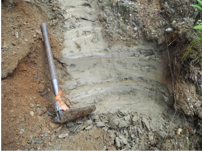
Figure 7. Lake deposits in gully north of Sherman Hollow Road. Bedded very fine sand and fine sand with widely spaced laminae of silty clay.
