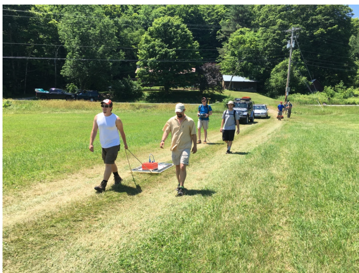
Figure 12: Ground-penetrating radar antennas (orange) being dragged across the floodplain of the North Branch valley.
