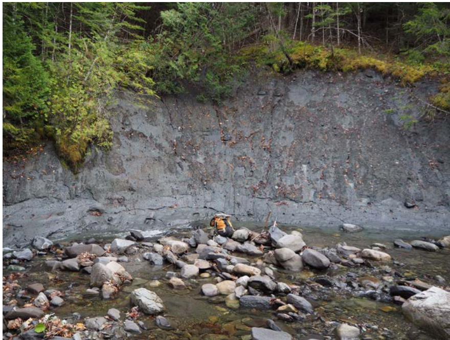
Figure 8. Exposure of dense silt till in landslide on Morrill Brook, Station JP602.
