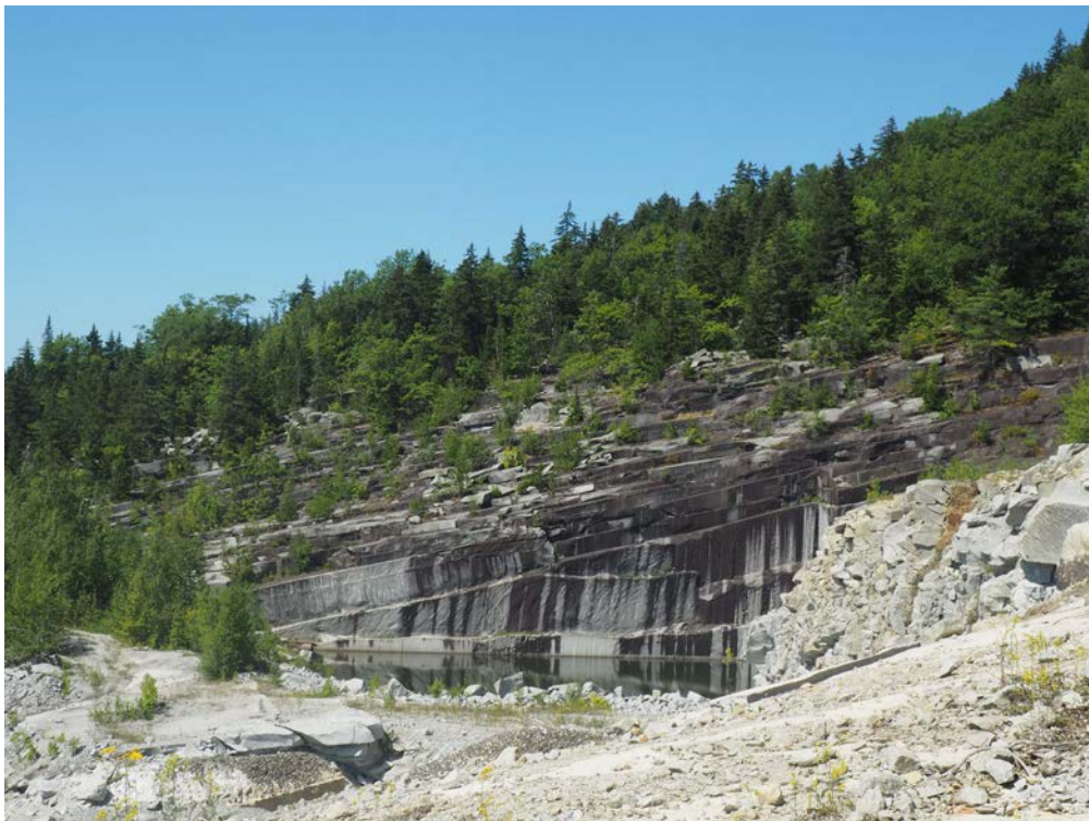
Figure 10. Flooded granite quarry hole on west side of Blue Mountain. Note prominent sheeting joints dipping west (left).
