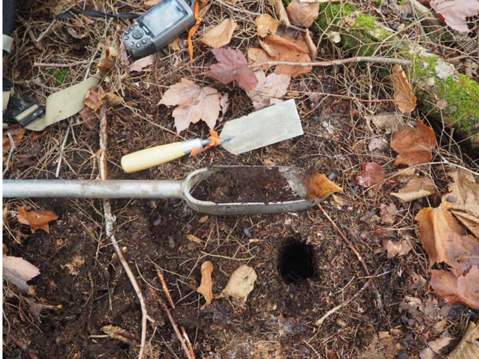
Figure 20. Spodosol developed on sandy glacial till. Note ashy gray leached (E) horizon below dark brown A horizon and above an orange-brown B horizon. Site is in hemlock woods.
