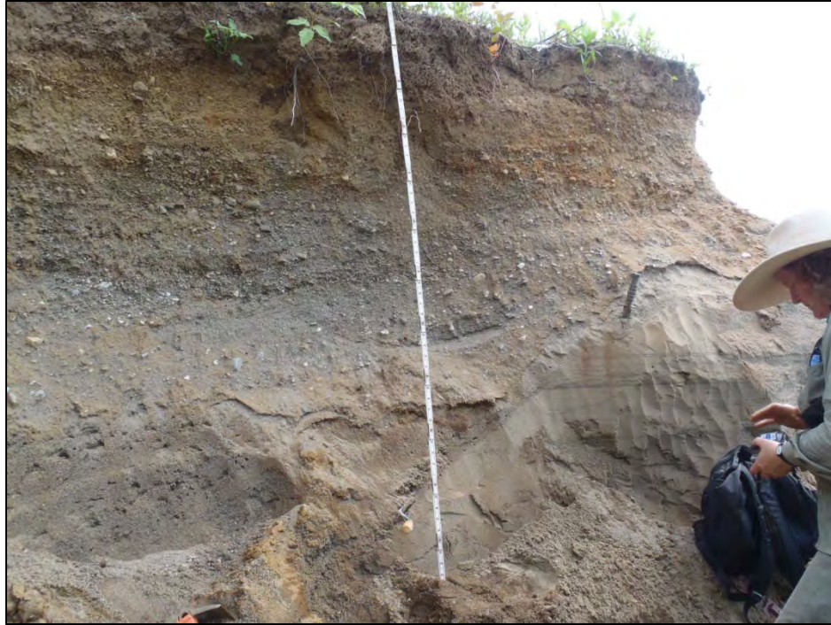
Figure 21. Fluvial sand and gravel over lacustrine fine sand at the top of the section. June 7, 2011.
