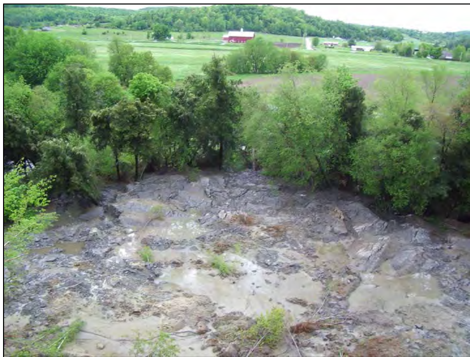
Figure 20. Looking down landslide at blocks of silt-clay in toe deposit on May 28, 2009.
