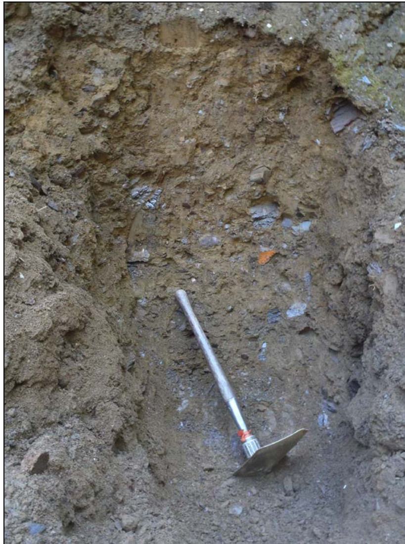
Figure 4. Closeup of a typical exposure of dense till. This site is from the Woodbury quadrangle to the west, but the till in the study area is quite similar in appearance. Site WO470, south of King Pond Road.
