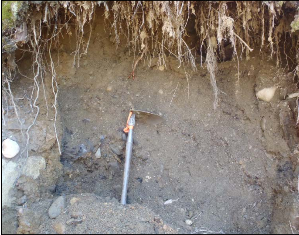
Figure 11. Ice-contact gravelly sand exposed in a small pit on the east side of an access road, north shore of Nichols Pond.
