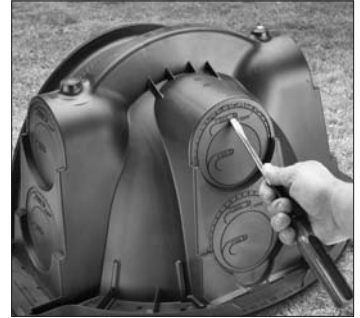
1. Start tear-out seal.
