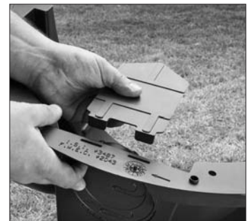
4. Install splash plate.
