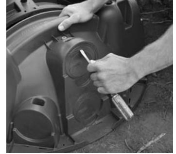
1. Start tear-out seal.
