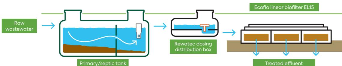
Figure 1.3.1 | Ecoflo linear EL15 biofilter system with gravity distribution
