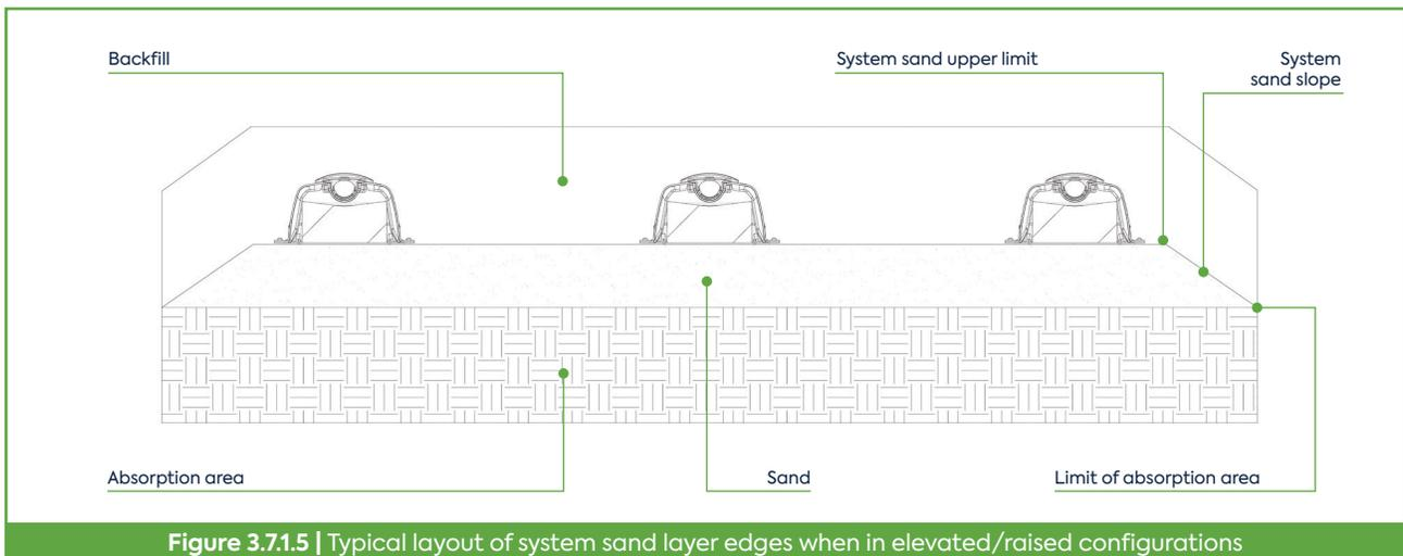
Figure 3.7.1.5 | Typical layout of system sand layer edges when in elevated/raised configurations
