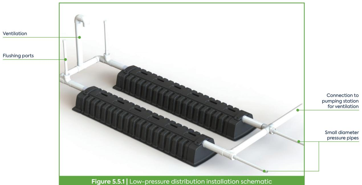
**Figure 5.5.1 | Low-pressure distribution installation schematic**
