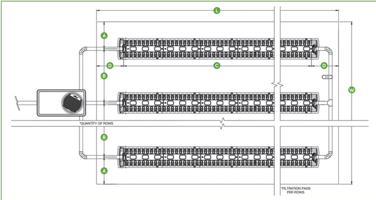
Figure 5.3.1 | Typical bed layout — Slope between 0 to 4%
