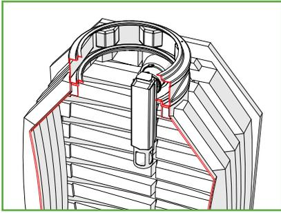
As per ANSI/NSF Standard 40 certification, the primary/septic tank must have a minimum effective capacity of 1.9 times the daily design flow. The tank must be rectangular in shape and/or composed of two rectangular tanks in series. It must comply with local regulations.
