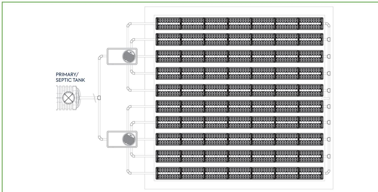
Figure 3.5.1.1 | Ten treatment lines installation fed by two Rewatec dosing distribution boxes
