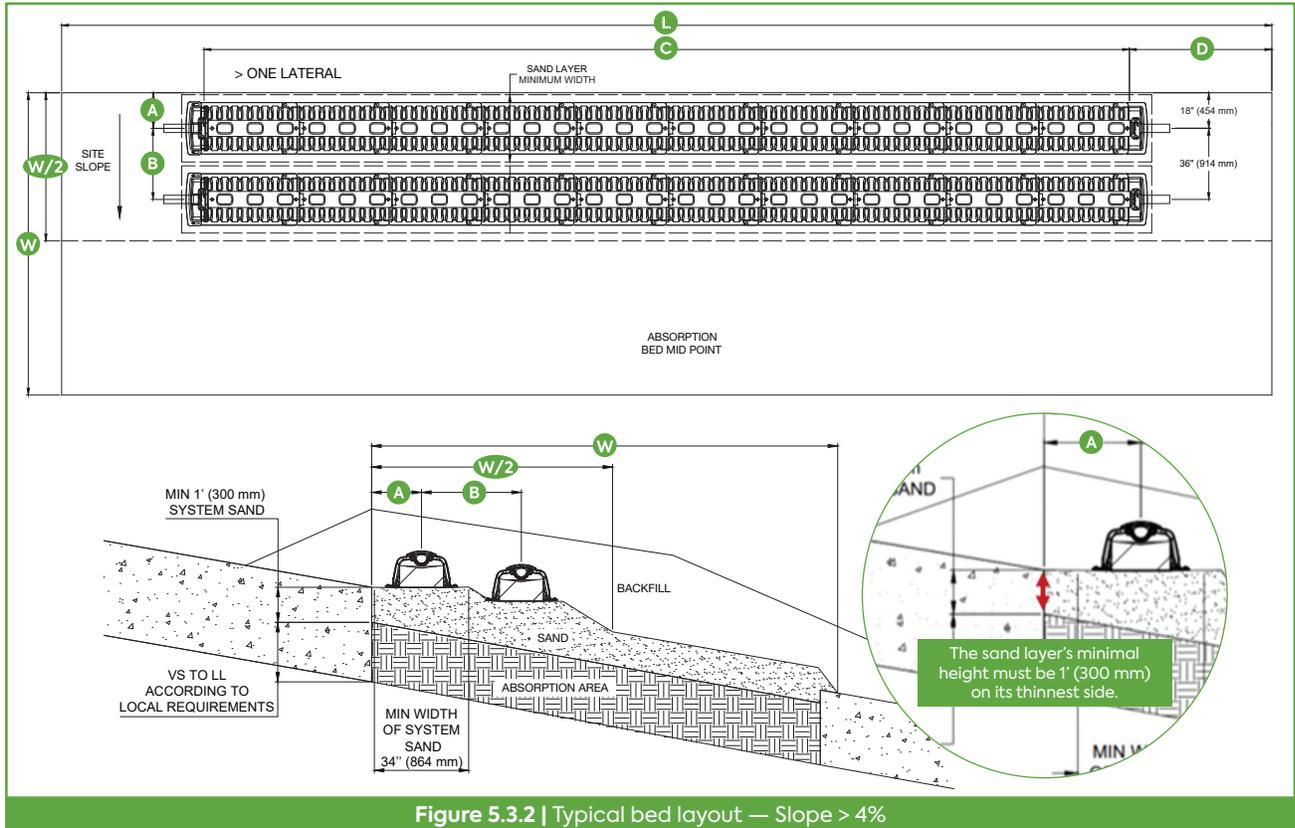
Figure 5.3.2 | Typical bed layout — Slope > 4%
