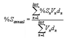
For gaseous fuel burned during the year the requirement is met if the annual average sulfur content is equal to or less than 0.05 percent by weight. The sulfur content of the gaseous fuel shall be determined by certifications provided from the fuel supplier certifying the sulfur content of the gaseous fuel that is delivered to the Facility.
