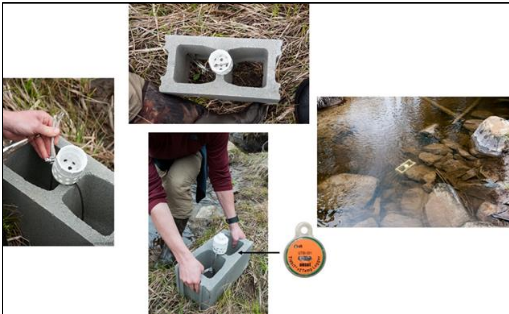
Figure 3.1.A Sensor deployment utilizing a cement block.
