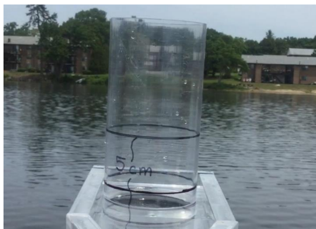
Figure 6.1.B Setting sectioning tube with 1 cm marking over stage. Water has already been siphoned off the top of the core.
