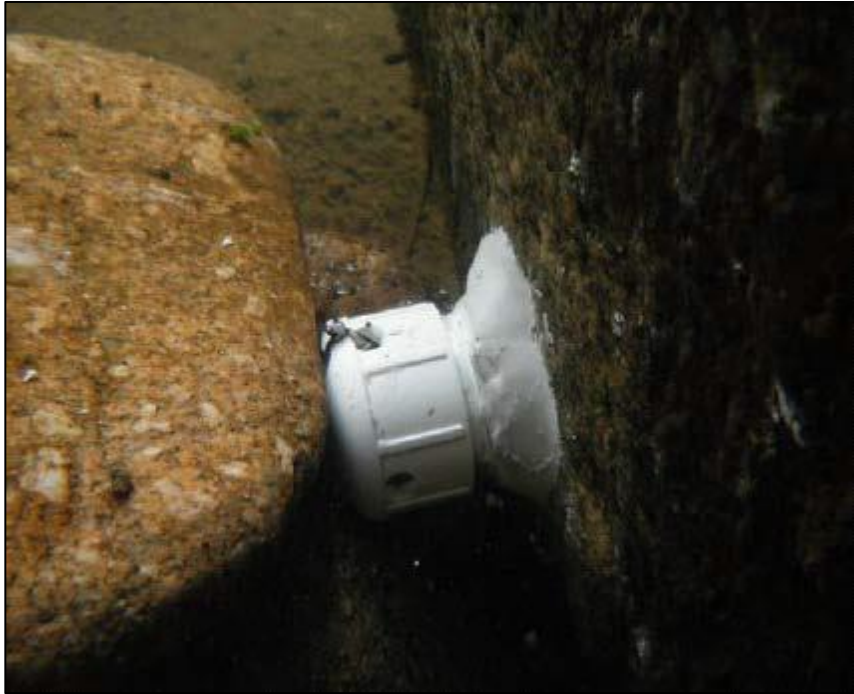
Figure 3.1.B Permanent water temperature logger deployment using in-stream substrate and epoxy.
