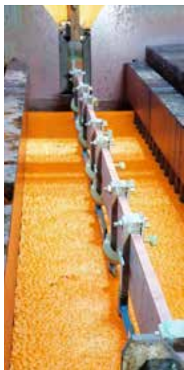
Image 1: Fumalock® foam blanket on bath surface of chrome plating bath
