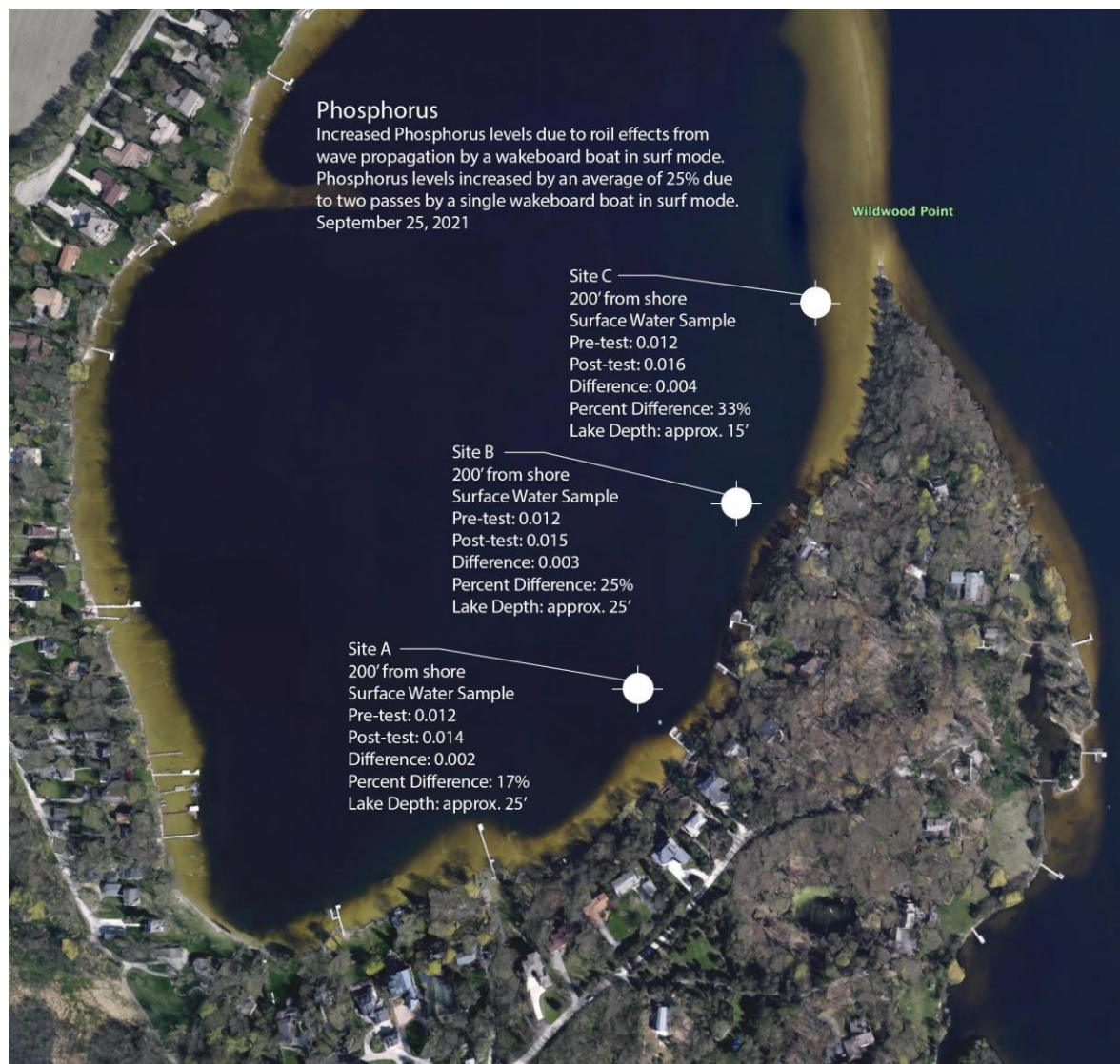
Figure 12 Increased Phosphorous Release Events Following Wake Board Boat in Surf Mode Operations, North Lake, Wisconsin Study (2021).
