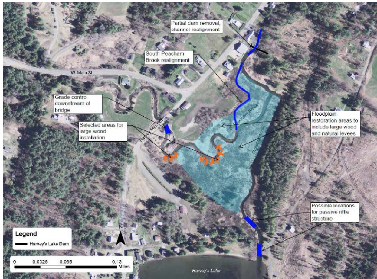
Figure 26. Preliminary design concept for Harveys Lake Dam removal (2018 Harveys Lake Design Concepts Report, Interfluv).
