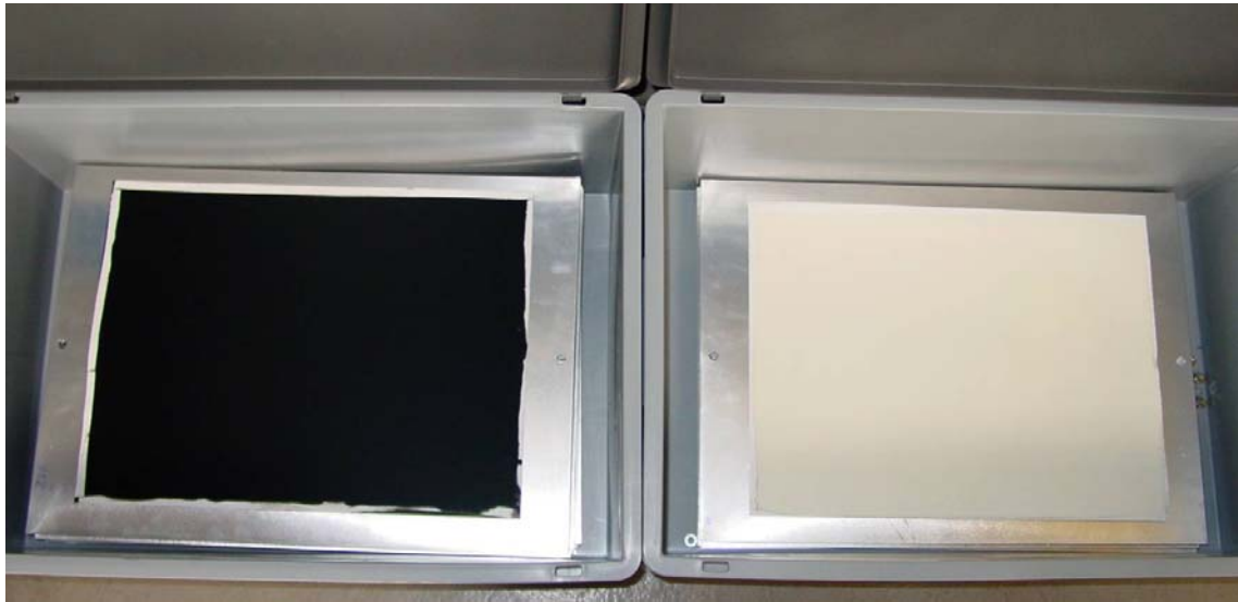
Fig. 5: Filters (300 mm x 400 mm) after particle sampling. Left from Diesel engine (filter loaded with 0.6 g particles), right from almost-complete wood combustion (filter loaded with 1 g particles).
