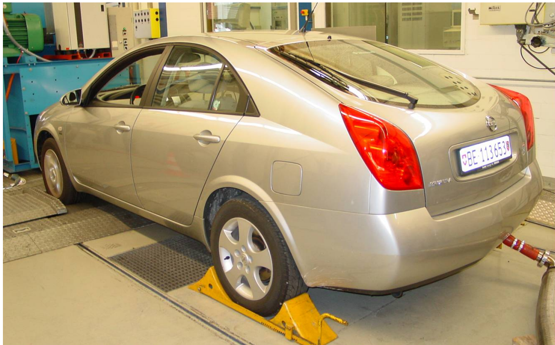
Fig. 4: Particle sampling from the exhaust gas of a Diesel car without internal particle filter according to Euro 3 emission standard (Nissan Primera 2003) on the test-bench at EMPA Dübendorf.
