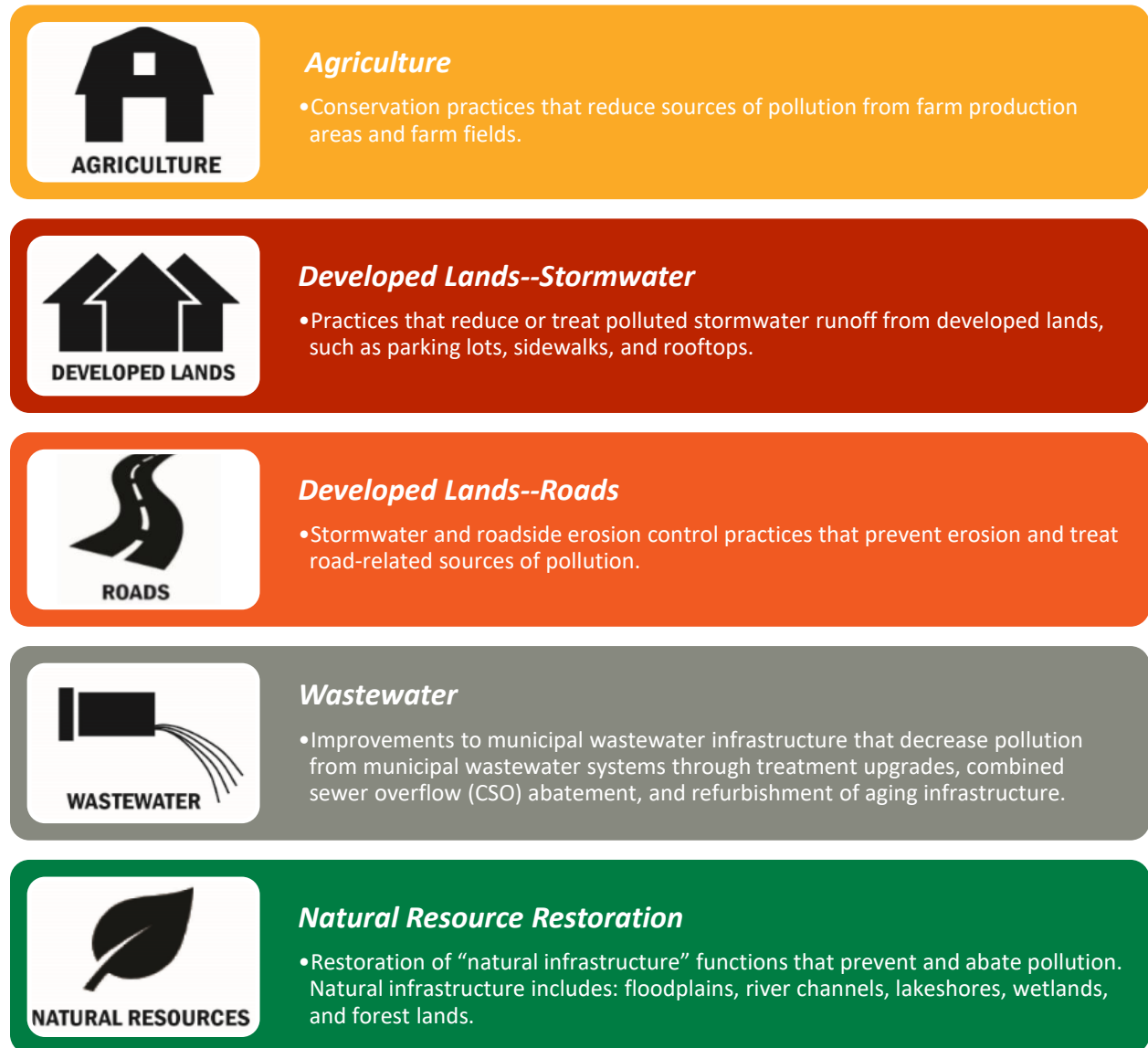
Figure 18. Land Use Sector Framework with practices used to enhance, maintain, protect, and restore water quality
