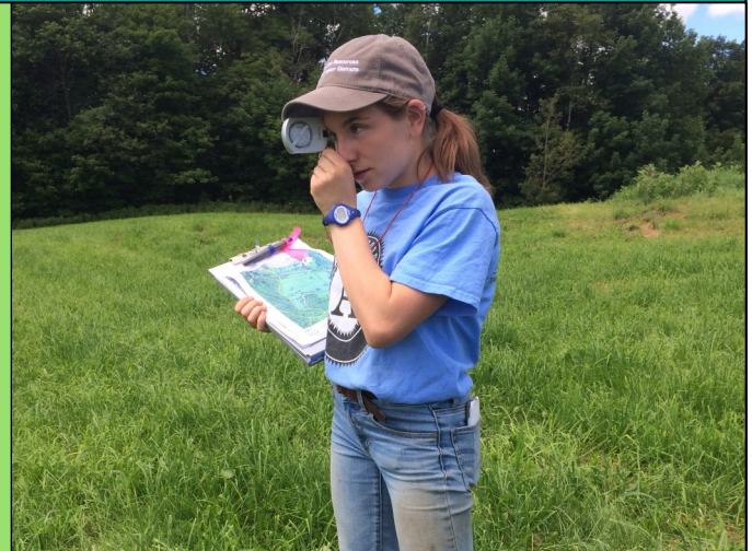
ECO Member Lindsay uses a clinometer to assist with determining the slope of an agricultural field.
