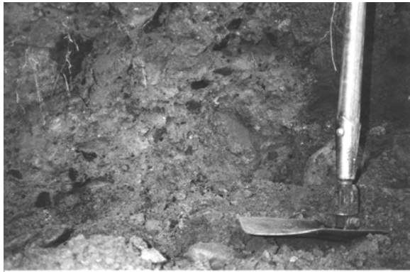
Figure 3.3 Highly compacted basal till.
