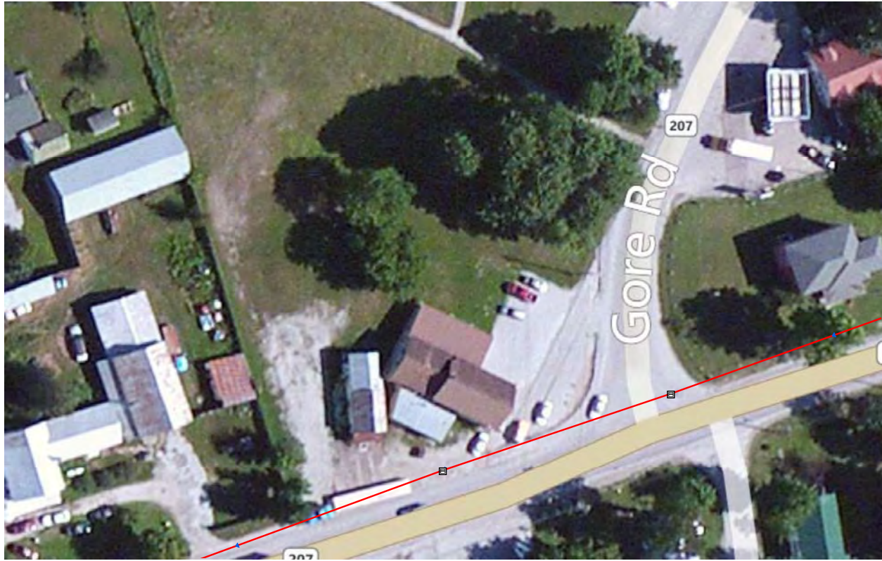
Figure 14. The Highgate Municipal Town Plan proposes the construction of a Park-and-Ride facility at the corner of VT-207 and VT-78. Soil conditions favor infiltration practices such as porous pavement at this site.
