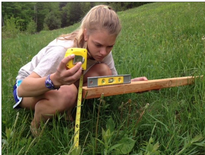
Once the board is level, from the bottom of the board, measure how many inches off the ground it is. This measurement is the Rise and the 50" board is the Run. The slope formula will give the percent slope.
