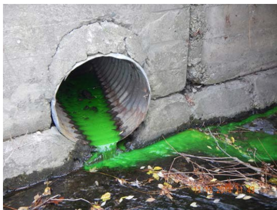
Dye indicative of raw sewage in stormwater outfall. This illicit discharge has been corrected since this photo was taken.
