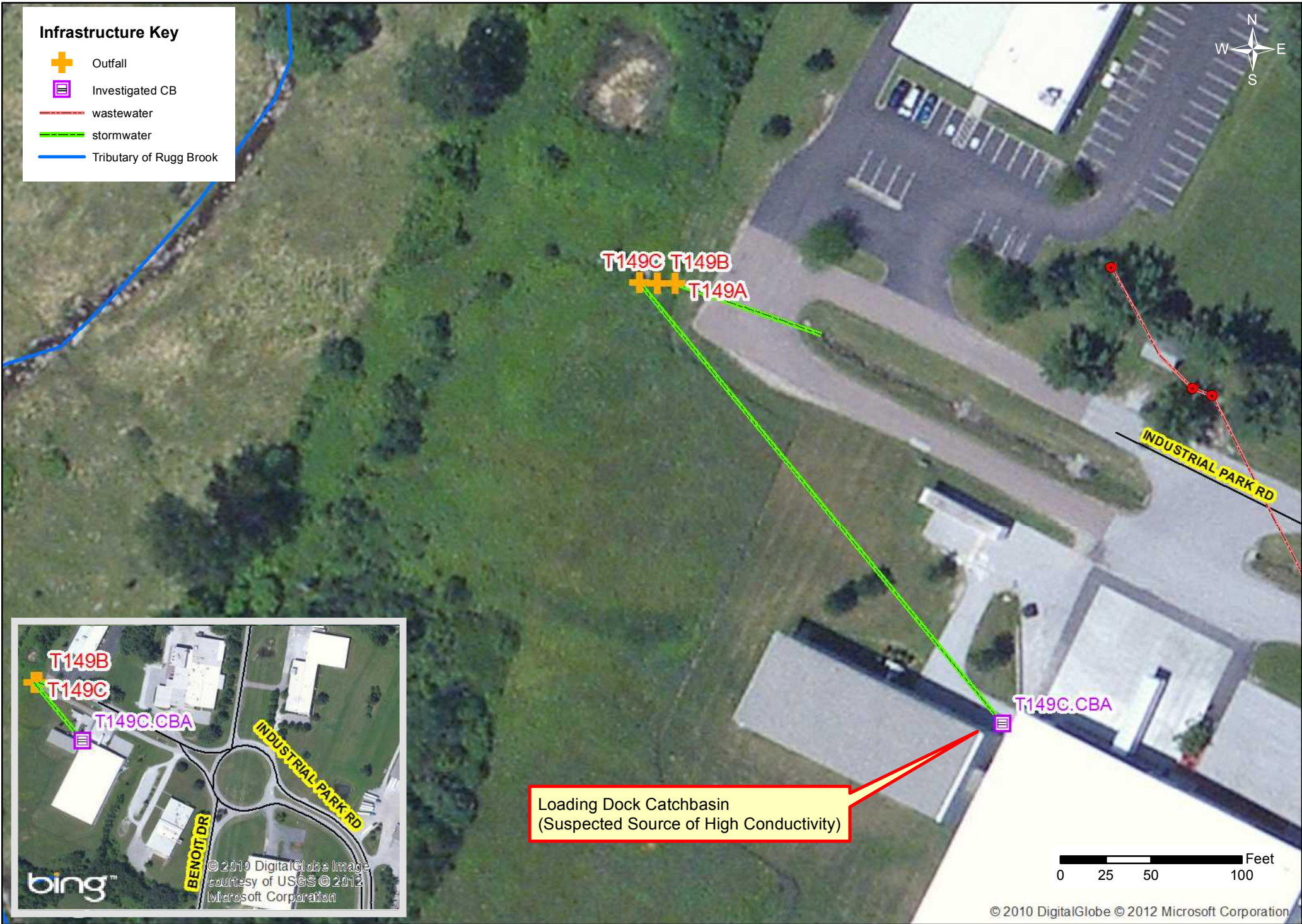
Figure 5-12: Problem Site Investigation for Outfall T149C
