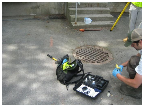
Figure 7: Ammonia Testing at Loading Dock Catch Basin (24.CBD) on June 8 th , 2012.
