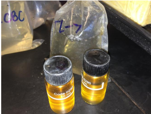
Figure 37: Reacted Samples from TL-7 Indicates High Concentration of Ammonia (> 5.0 mg/L)
