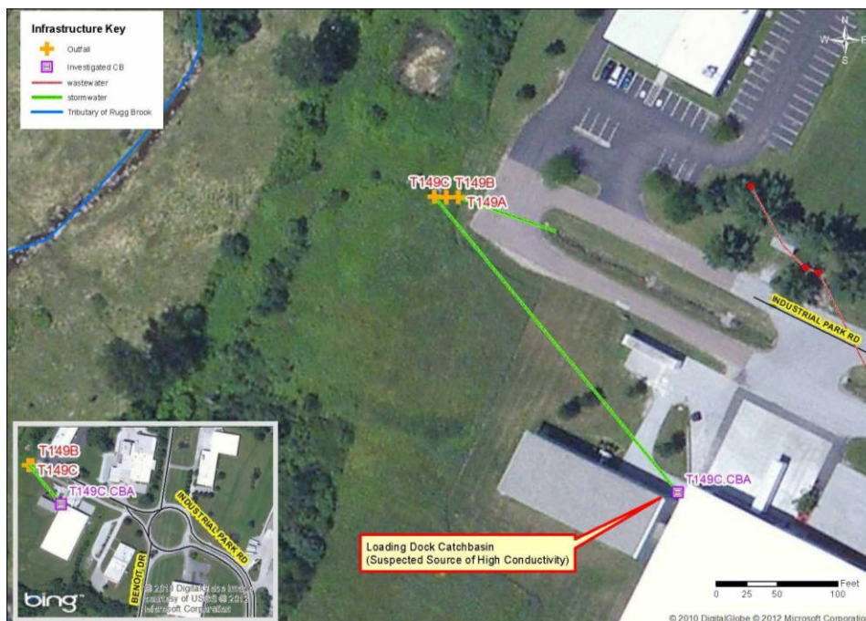
Figure 32: Outfall T149C Drainage System
