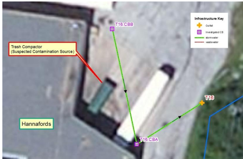
Figure 28: Outfall T16 Drainage System
