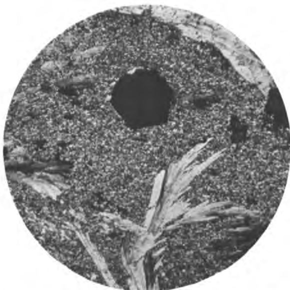
Figure 20. Photomicrograph ( \times 18 ) of a dark hornblende-rich band from the Gile Mountain formation showing plumose, porphyroblastic hornblende and idioblastic garnet in a very fine groundmass of plagioclase, quartz, and iron ores. From northeast of Kirby Pond (H0211; see Fig. 15).
