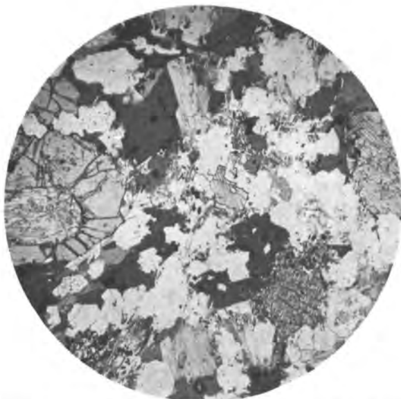
Figure 61. Photomicrograph ( \times 18 ) of sillimanite-garnet hornfels, showing idiomorphic sillimanite (one surrounded by garnet) containing inclusions of quartz, biotite, and muscovite; some fibrolite. The other minerals are biotite, muscovite, a little microcline, oligoclase, and iron ores. From Lees Hill (I2725).
