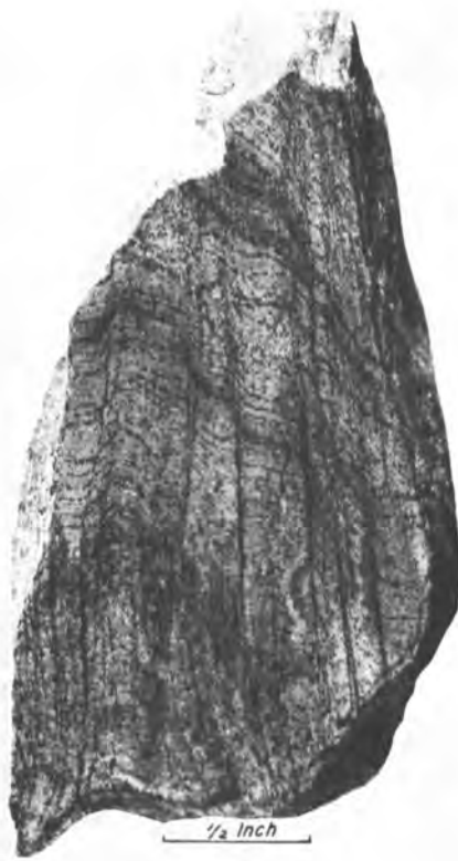
Figure 41. Photograph of polished surface of Wait's River quartzose phyllite showing shear fold in bedding schistosity ( S_1 ) caused by slippage on S_2 cleavage. Biotite is aligned in both S_1 and S_2 . From west of Sugar Hill (G3009).
