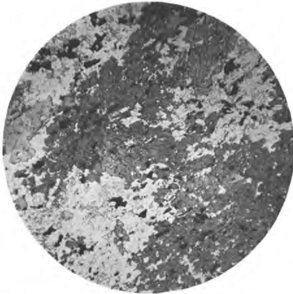
Figure 12. Photomicrograph ( \times 18 ) of Waits River amphibolite showing poikiloblastic hornblende in a groundmass of plagioclase, quartz, calcite, apatite, chlorite, and iron ores. Northwest of Graves Hill (G0930).
