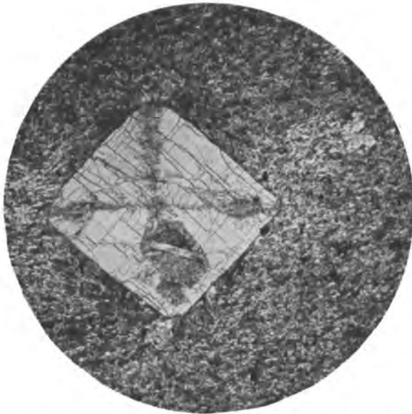
Figure 19. Photomicrograph ( \times 18 ) of Gile Mountain andalusite hornfels showing idioblastic andalusite (var. chiastolite) with inclusions of opaques, quartz, biotite, and muscovite in a fine groundmass of quartz, biotite, muscovite, and opaques. From East Mountain (F2947).
