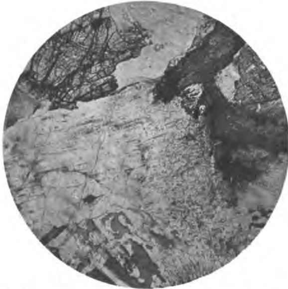
Figure 64. Photomicrograph ( \times 18 ) showing an andalusite porphyroblast with inclusions of kyanite (top left), a kyanite porphyroblast (top right), and biotite, in part altered to fibrolite (right). The large area in the center is partially kaolinized oligoclase with inclusions of fibrolite; quartz with fibrolite inclusions is also present. Xenoblastic staurolite occurs elsewhere in the slide away from the quartz-oligoclase vein. Muscovite is abundant in the vein and elsewhere. From east of Route 114 (B1848).
