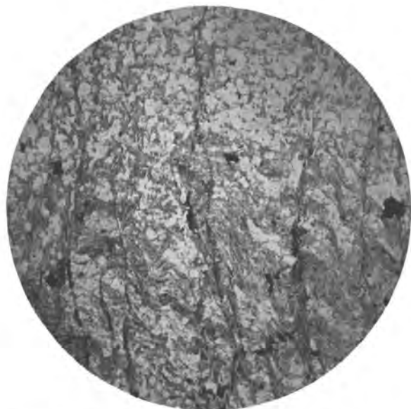
Figure 32. Photomicrograph ( \times 18 ) of banded phyllite, with minor calcite, from the transition zone between the Waits River and Gile Mountain formations, showing folded sericite schistosity ( S_1 ) cut by S_2 cleavage, biotite porphyroblasts (some lying parallel to S_2 ), and opaques in pelitic band (lower area). Note that S_2 surfaces are also developed in the quartzose band (upper area). From south of East Haven village (E1651).
