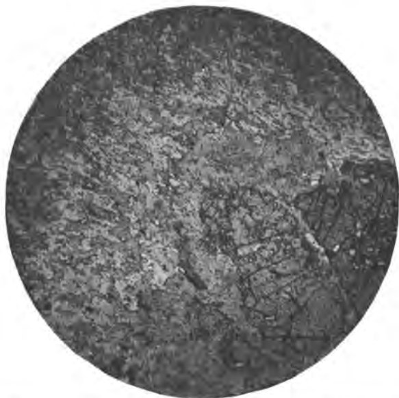
Figure 66. Photomicrograph ( \times 18 ) of staurolite-garnet-chlorite schist, showing poikiloblastic garnet (right) associated with poikiloblastic staurolite (below garnet), which is surrounded by muscovite aggregates and chlorite porphyroblasts. The groundmass is composed of chlorite, quartz, and sericite aligned into a wavy schistosity; rare green biotite and tourmaline are also present. Note "halo" around garnet and staurolite poikiloblasts where groundmass chlorite is almost absent. From northeast of Lyndonville (G0930).
