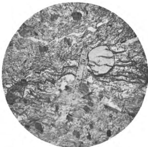
Figure 65. Photomicrograph ( \times 18 ) of staurolite-garnet schist, showing idioblastic staurolite and garnet with traces of relict wavy schistosity. Biotite porphyroblasts are abundant; chlorite porphyroblasts also occur (center). The groundmass is composed of quartz, sericite, and iron ores. From the Moose valley (F1519).
