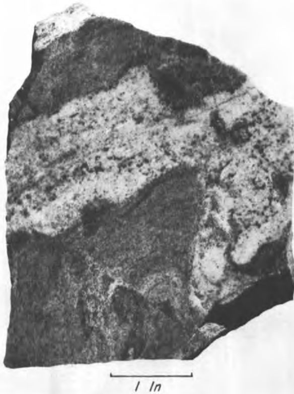
Figure 23. Photograph of a hand specimen of migmatite from outcrop on road to the summit of Burke Mountain (H1156).
