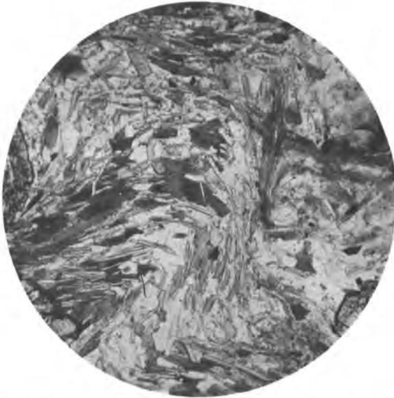
Figure 67. Photomicrograph ( \times 44 ) of staurolite-garnet-sillimanite hornfels, showing garnet (bottom left), staurolite (left and bottom right), and poorly-oriented biotite porphyroblasts in a groundmass of quartz, sericite, opaque dust, and scarce apatite and tourmaline. Fibrolite (right) occurs as tufted aggregates after biotite. From Victory (H3410).
