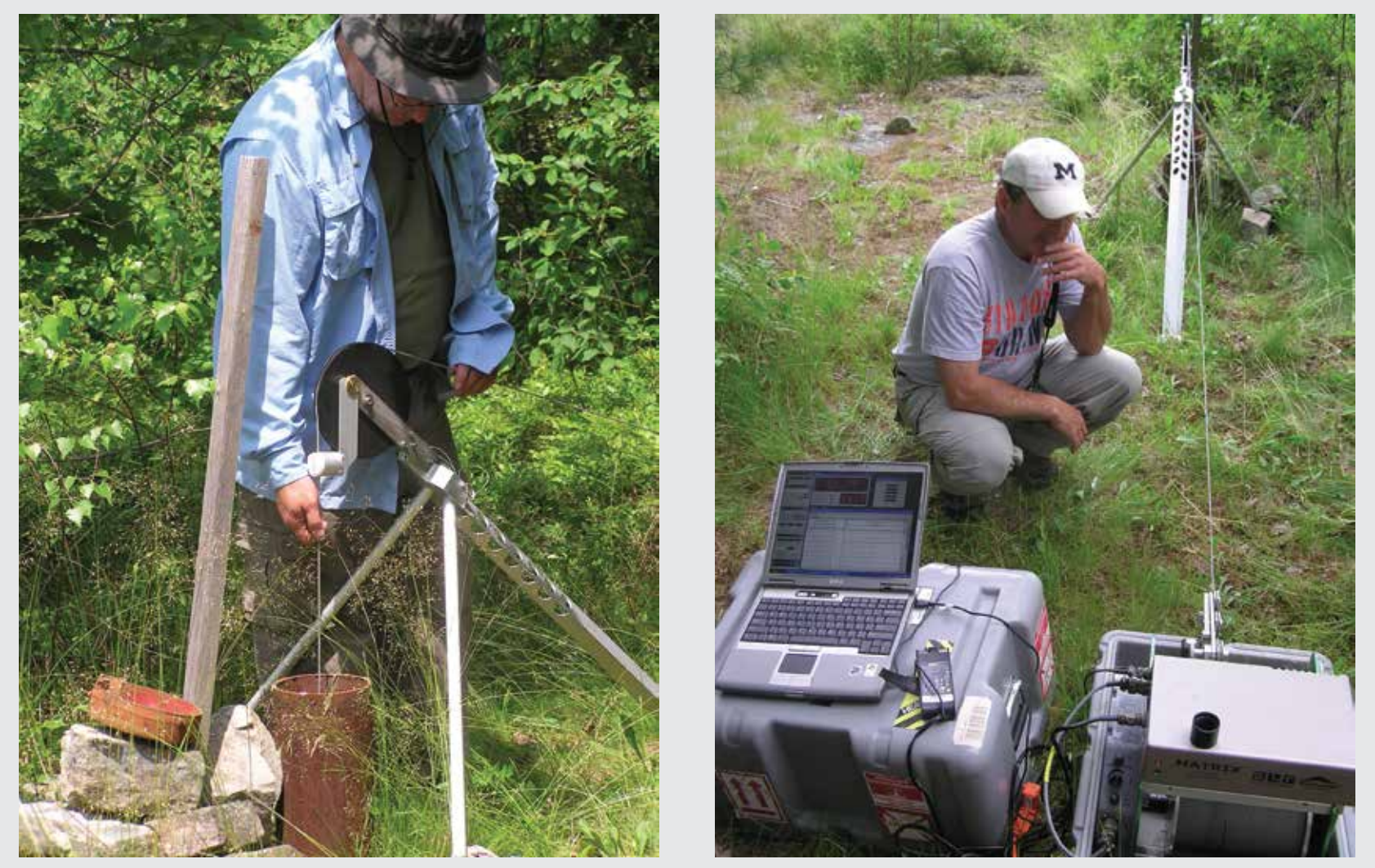
Left: Ed Romanowicz checking tension on the cable at the Altona Flats well field near Plattsburgh, New York. Right: Dave Franz inspecting the full logging set-up.
