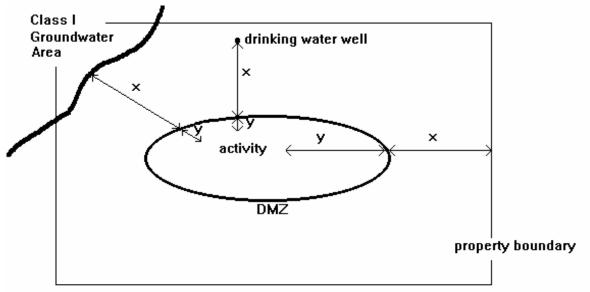
$\times$  + y = the total distance from the activity to the compliance point  $\times$  must be greater than or equal to 2/3 of the total distance y must be less than or equal to 1/3 of the total distance
